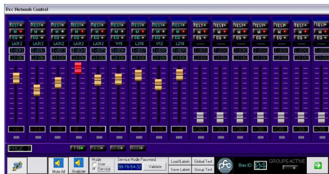
master screen enables to level, test, analyse, equalise and mute each cabinet and all groups
